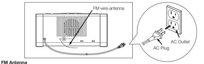
Unwind the FM wire antenna, located on the back cabinet, and extend it to its full length for best FM reception.
